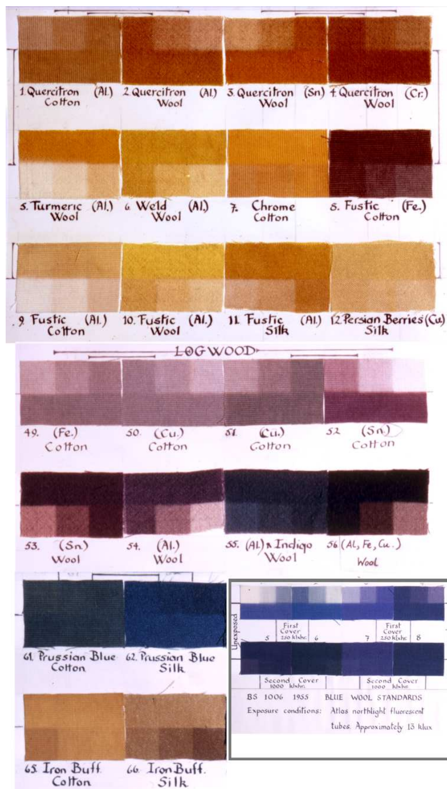
Figure 4: A continuation of figure 1 in the main text. This picture shows more dyes than were displayed (in monochrome) in the original article. The blue wool standards are shown in the inset at bottom right.
