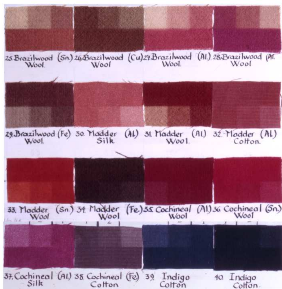
FIG. 1. Some of the faded specimens. The rectangular areas are unexposed. The three square areas on each specimen have been exposed to 7.8, 36 and 91 million lux hours of light from Atlas "Northlight" fluorescent tubes. In all the dyeings illustrated here the palest area has received the greatest light dose. The GS difference between exposed and unexposed dye is written on the unexposed part.
